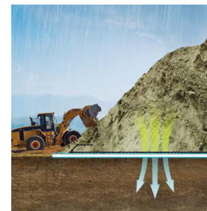
In-situ containment of contaminated soils
